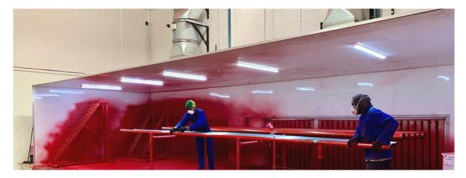
IMS Pipe Fabrication is the only fire sprinkler pipe manufacturer in the Western Cape with a fully equipped spray booth specially designed for precise paint application to steel pipe work. All pipe work leaves our factory with the correct paint primer and enamel coating to required micron thickness.
